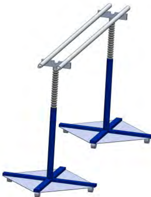
An example of a conductor cover that is tested using a stand CTS-1
