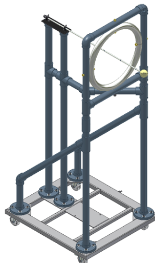
SW-1 Voltage and Phase Indicator Testing stand
